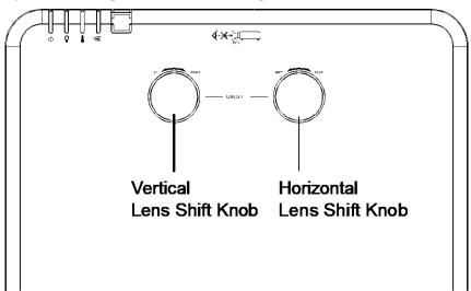
The Lens Shift feature provides a lens shift function that can be used to adjust the position of the projected image either horizontally or vertically within the range detailed below.
