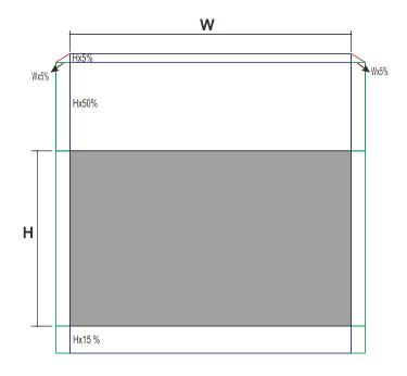
When W and H at 0% offset position The max. H up shift=Hx55% The max. H down shift=Hx15% The max. W shift=Wx5% When max. W shift is Wx5% max. H shift=Hx50% When max. H shift is Hx55% max. W shift=Hx0%
