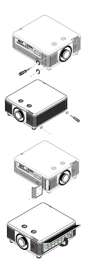
**3.** Lift the filter from the filter cover.
