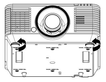
**2.** To lower the level of the projector, lift the projector and twist the adjusters clockwise.
